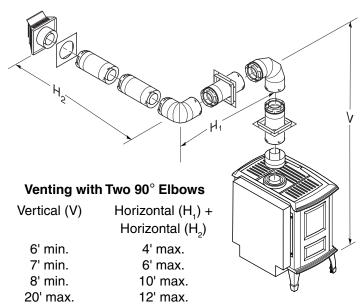
Figure 30 - Horizontal Termination Configuration for Venting Using Two 90° Elbows with Termination at 90° with Stove
